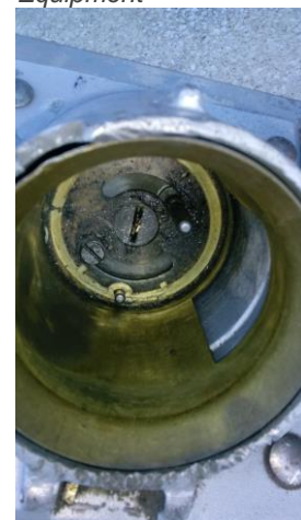
Figure 6 - Broken Key in Collections Equipment
